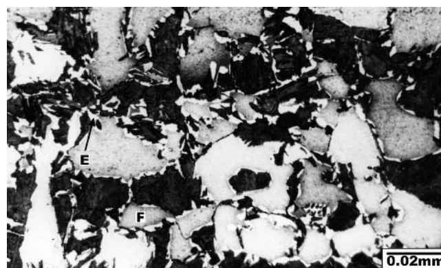
Fig. 1 Microstructure of dual-phase steel after intercritical annealing at 780 °C and then quenching in hot water shows the effect of alkaline chromate etch. M = martensite, F = old ferrite, and E = epitaxial ferrite
